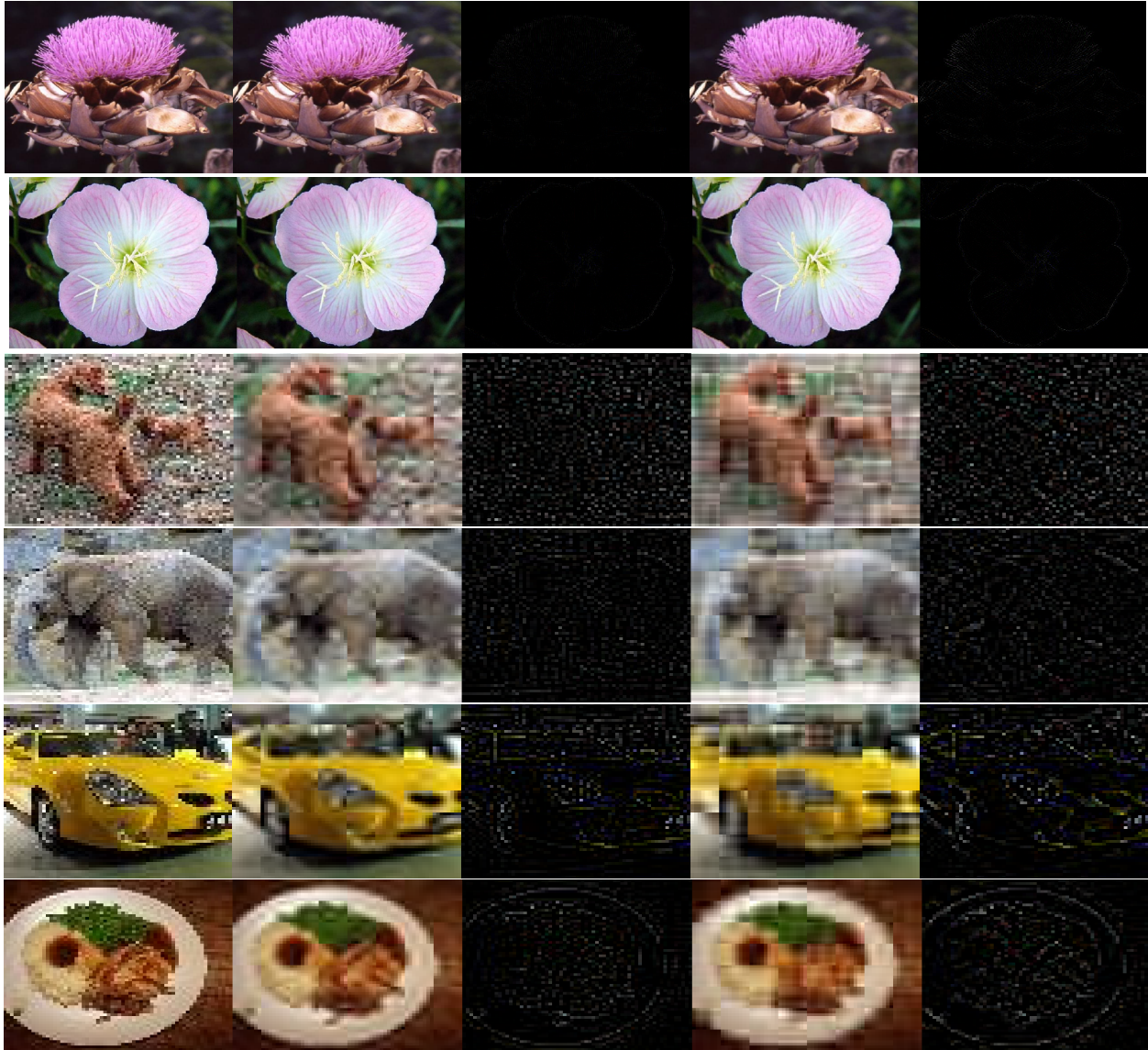
Figure 3.9: Visualization of the effect of removing frequency channels on RGB domain. From left to right column: (1) original image; (2) IDCT_{24} : reconstructed image after removing frequency channels as in [27] and keeping only 24 channels; (3) image-IDCT_{24} : removed information in RGB domain; (4) IDCT_{18} : reconstructed image with our channel selection strategy; (5) image-IDCT_{18} : our removed information in RGB domain. Images from the first 2 rows are from Flowers-102 dataset and the rest rows are from the Tiny-ImageNet dataset.
