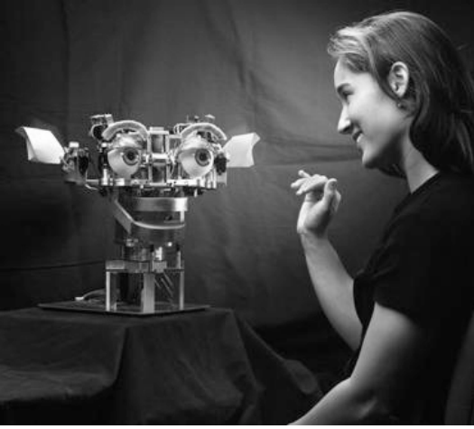
Figure 1: Kismet, a robot designed to interact socially with humans. Kismet has an active vision system and can display a variety of facial expressions.
